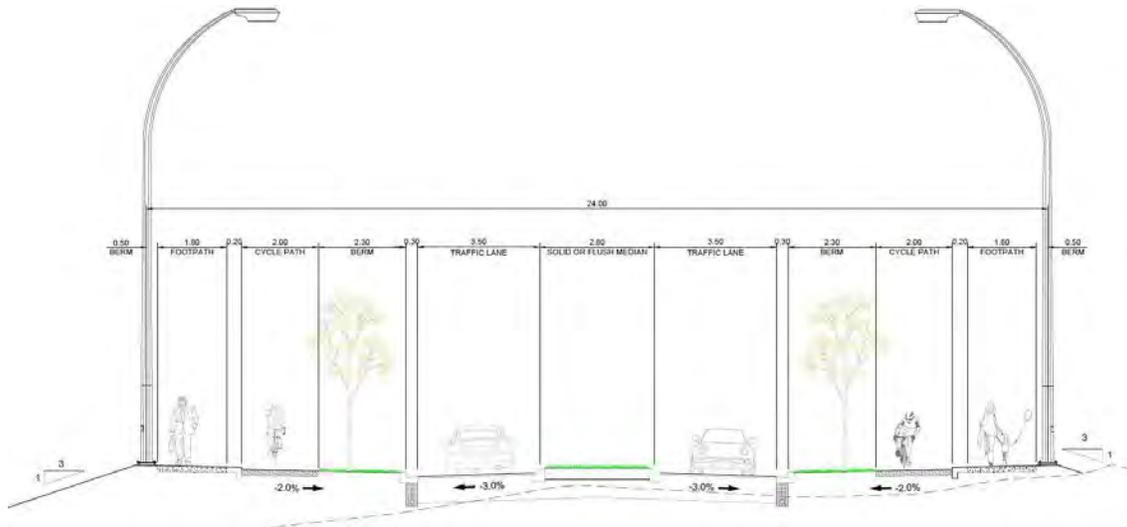
**Figure 5: Typical Cross Section for Ponga Road included within the Drury Arterial Network DBC**
