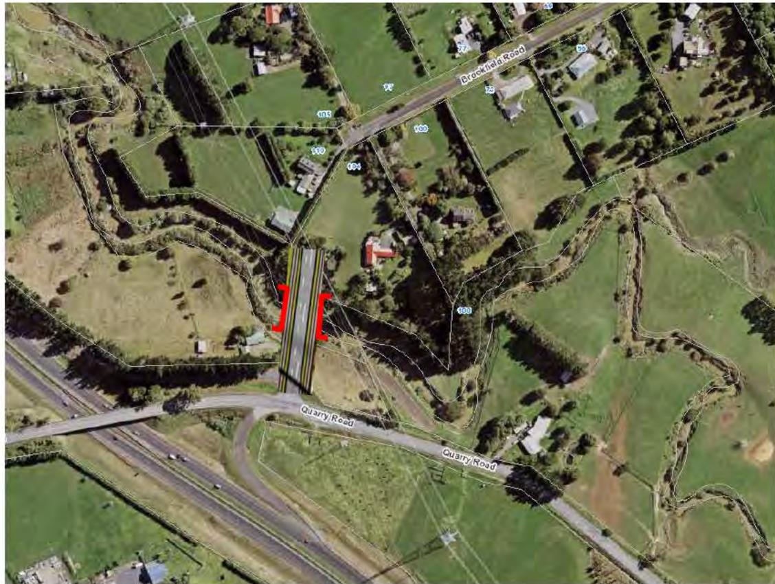
The total length of road has been measured to be 120m, including a 50m section of new bridge (18m wide). A new signalised intersection would be provided at the Quarry Road intersection.
