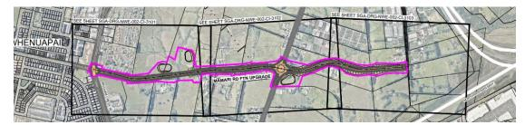
The project road is approximately 1.8 km and culminates at Northside Drive. It involves an upgraded intersection at Mamari Road, an over bridge over a stream and a two lane roundabout at the intersection with the New Speddings Road.
