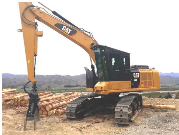
Figure 8: Typical forestry excavator (non-self-levelling) with grapple on a 'high and wide' carrier.
