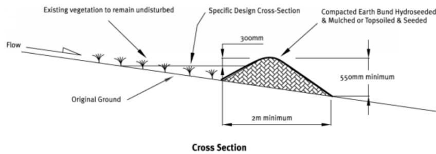
Figure 16: Cross-section of clean water diversion
