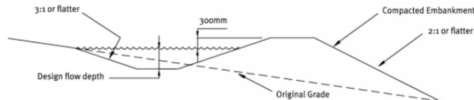
Figure 18: Cross-section of a dirty water diversion
