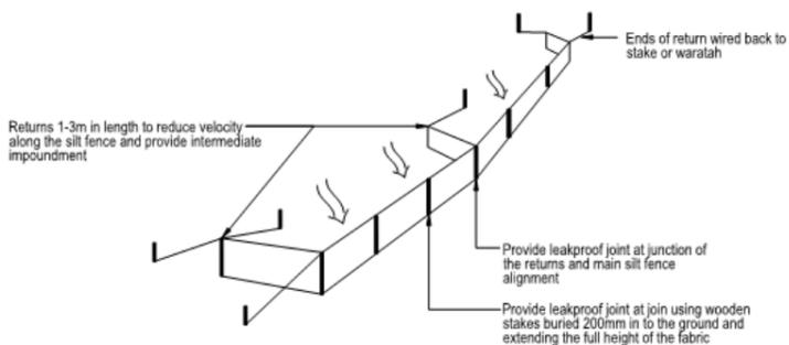
Silt fence with returns and support wire
