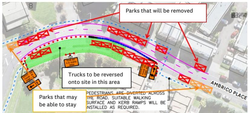
A two metre hoarding surrounding the site will be installed between early-April and mid-May. The hoarding forms a noise wall that will minimise construction noise. Noise will be monitored throughout the project to make sure it remains within allowed limits.
