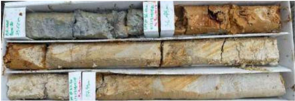
**Figure B12** Example of in-situ 'blocks' of cross-bedded Awhitu Formation within Ancient Colluvial/Alluvial soils, from BH-M06: 36.45-38.2 mbgl
