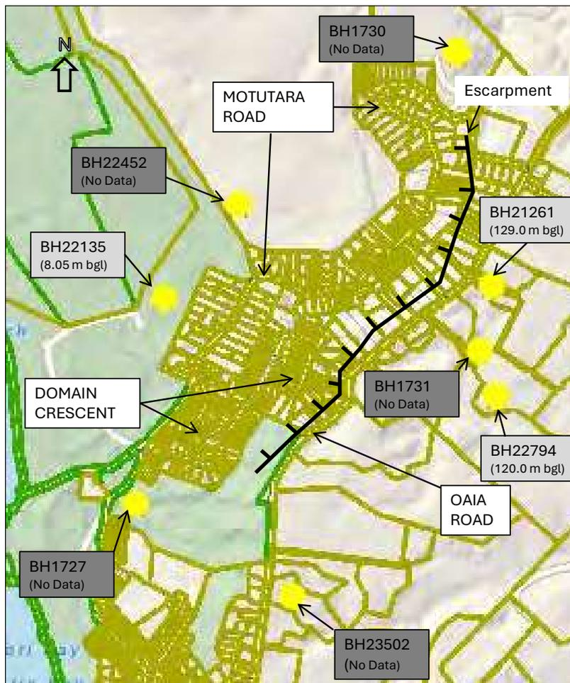
Figure B22 Historical well location plan with water level, where known (measured between 2004 and 2007). Supplied by AC.
