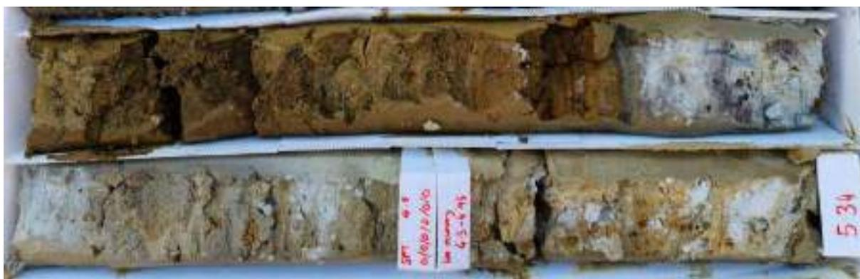
**Figure B11** *'Ancient Colluvial/Alluvial' soils recovered from BH-M07: 3.65-5.34 mbgl*
