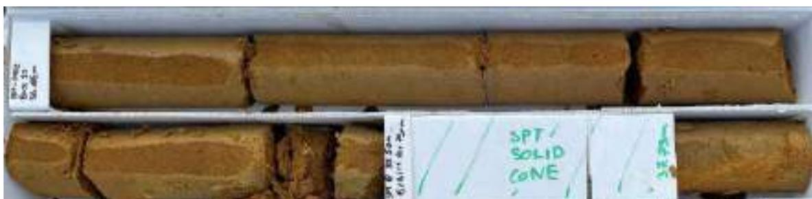
**Figure B18** *Example of Awhitu Formation Cemented very weak Sandstone, oxidised, from BH-M02 36.65-37.5 mbgl*
