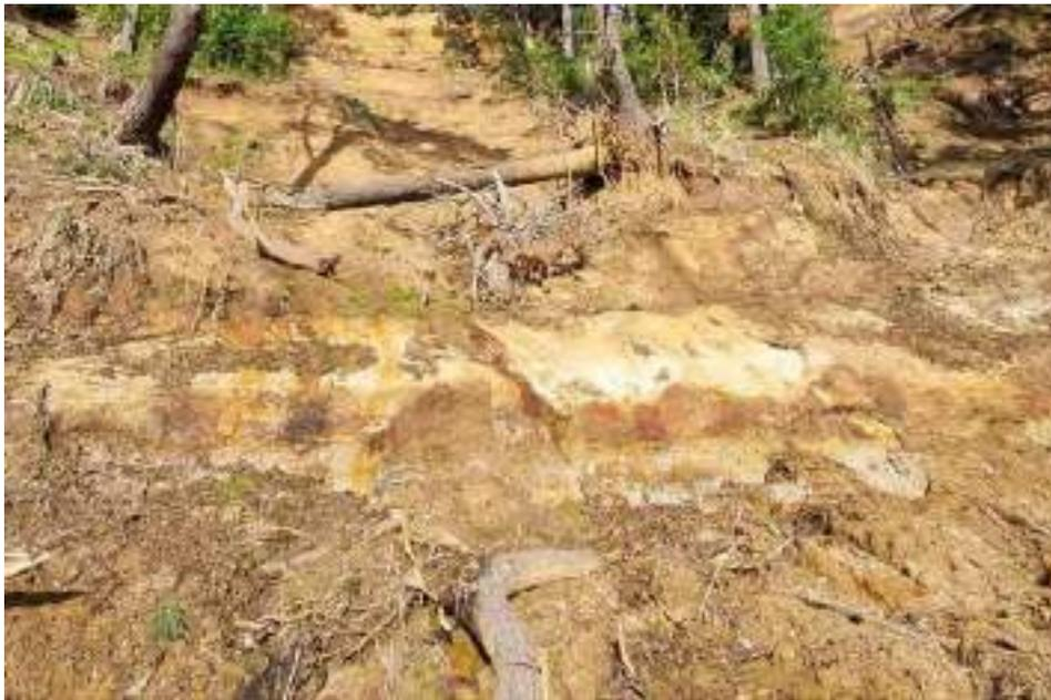
**Figure B16** *Outcrop of Awhitu Formation – Less Cemented Sands, layer of finer grained material (silt, clay). Approximate thickness 1 m.*
