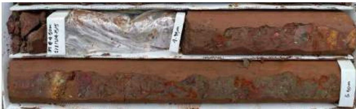
Figure B19 Example of Nihotupu Formation Residual Silt and Clay, from BH-M04 3.95-5.90 mbgl
