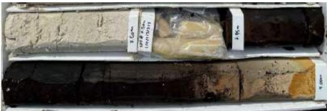
**Figure B17** *Example of layer of peat/organic soil within Awhitu Formation Less Cemented and Cemented Sandstones, from BH-M02, between 7.95 8.75 m bgl.*
