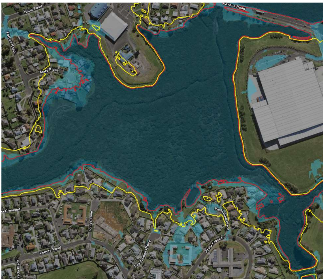
Figure 1-2 3m (red) and 4m (yellow) contour lines (AVD-46)
