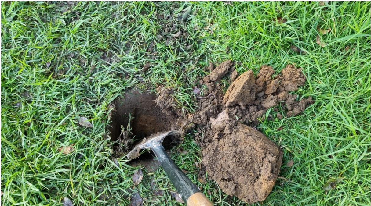
**Figure 13. Typical results of test pitting showing a mixed pale brown/orange clay**
