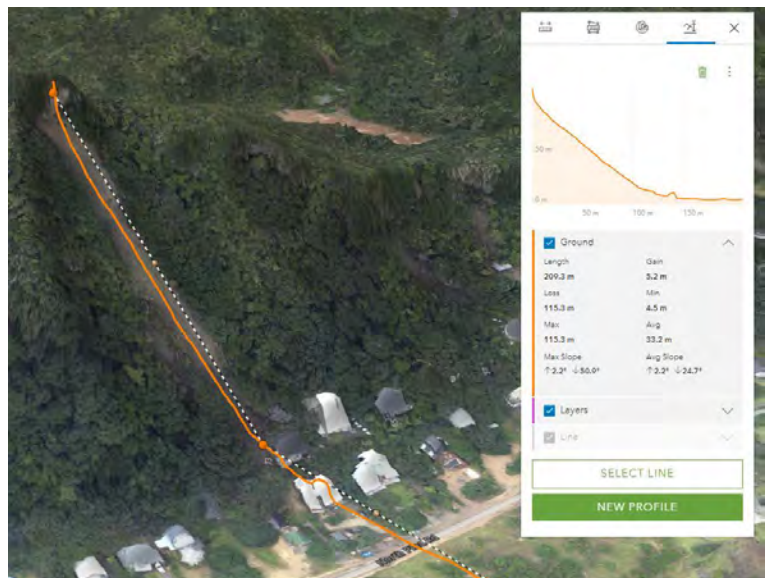
Figure 1: the profile of a landslide in North Piha from the Digital Elevation Model
