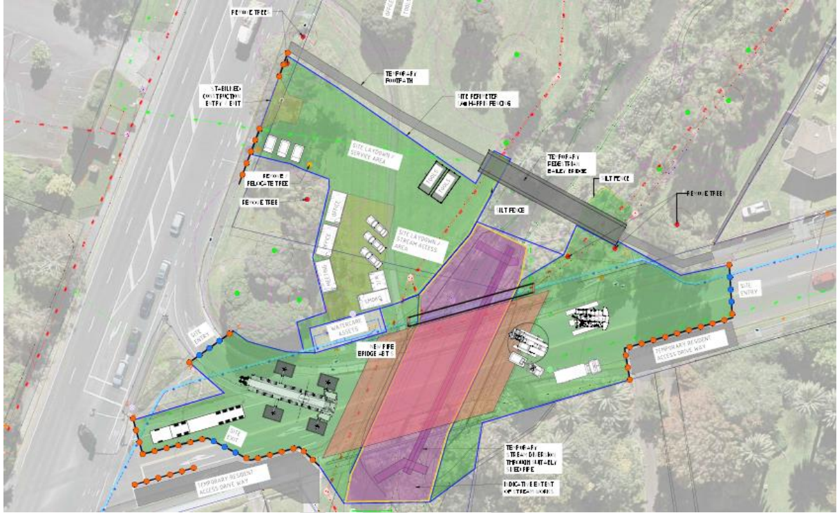
Figure 2: Extent of works for Te Ararata Flood Resilience Works – Walmsley Road Bridge Replacement.
