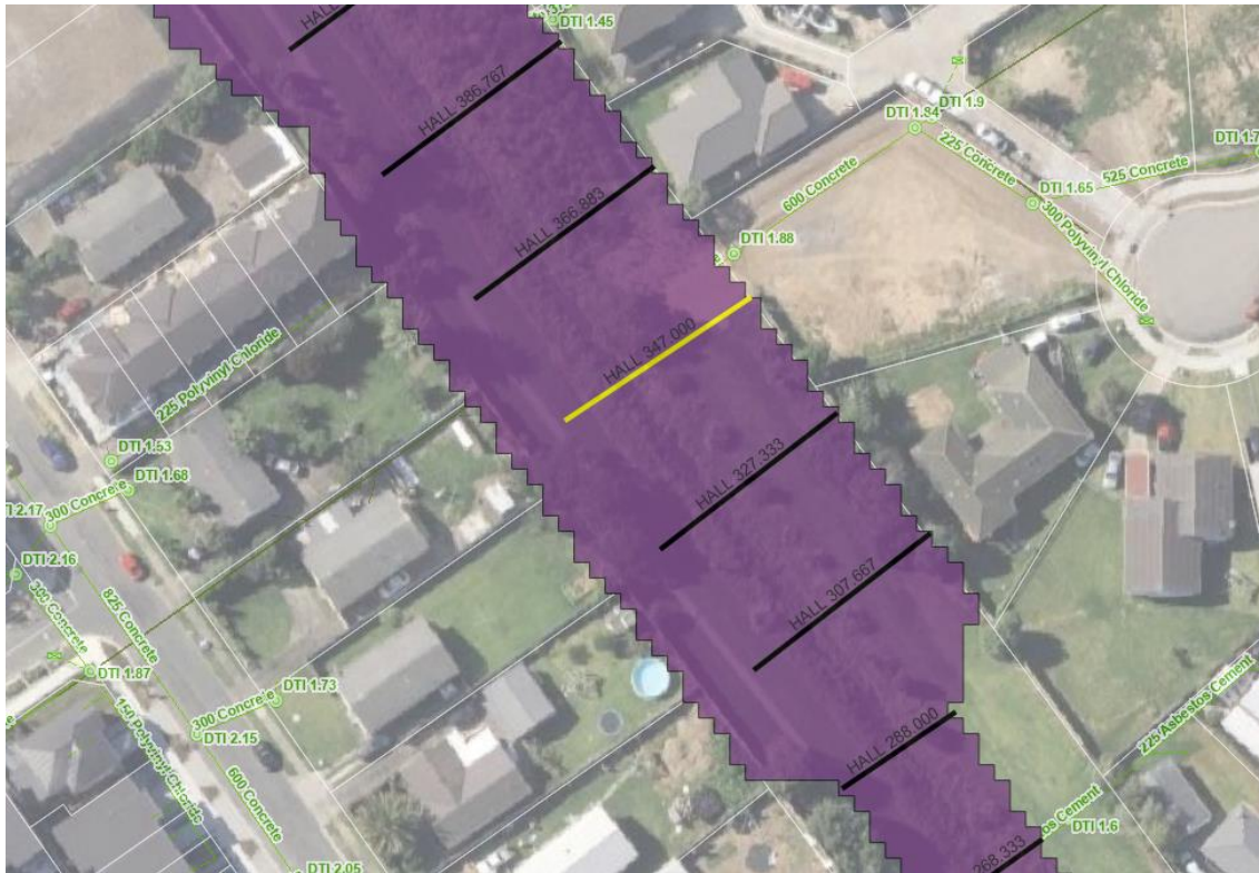
Figure 3.1: Te Ararata model – Example of old 1D cross sections not matching 1D extent from provided LEAD model.
