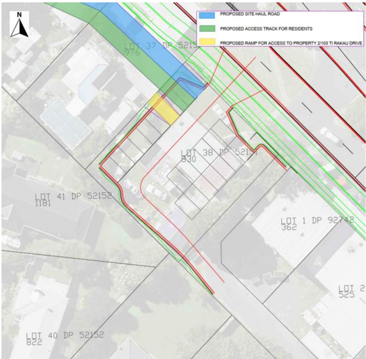
Figure 90: 103A Ti Rakau Dr temporary access
