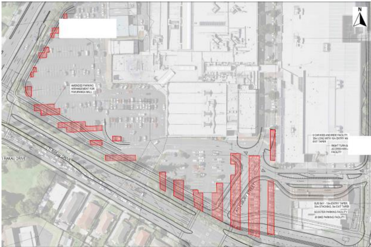
Figure 86: EB2 Ti Rakau Drive effects on parking at Pakuranga Plaza
