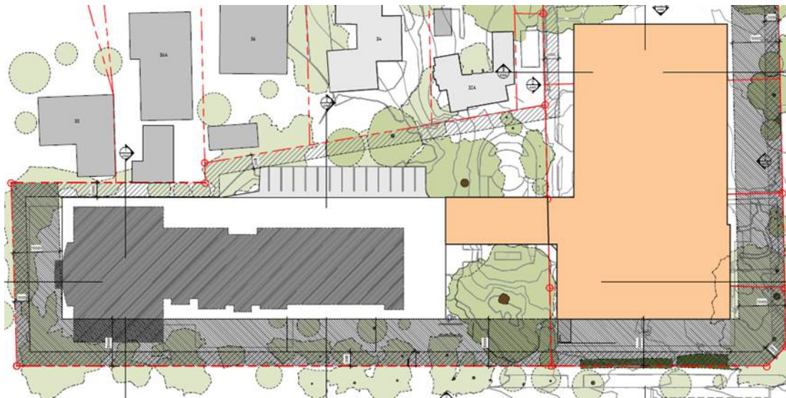
Figure 1: Excerpt from Babbage Civil Engineering report, drawing A920 (rev C) showing the proposed ground floor extent. An outline is shown extending over the existing hospital footprint and this has been assumed within the proposed basement excavation volume (less the current basement).
