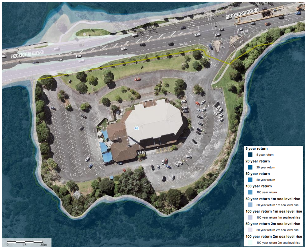
Figure 5: Coastal inundation risk to 48 Esmonde Road (Source: Auckland Council Geomaps 3 )
