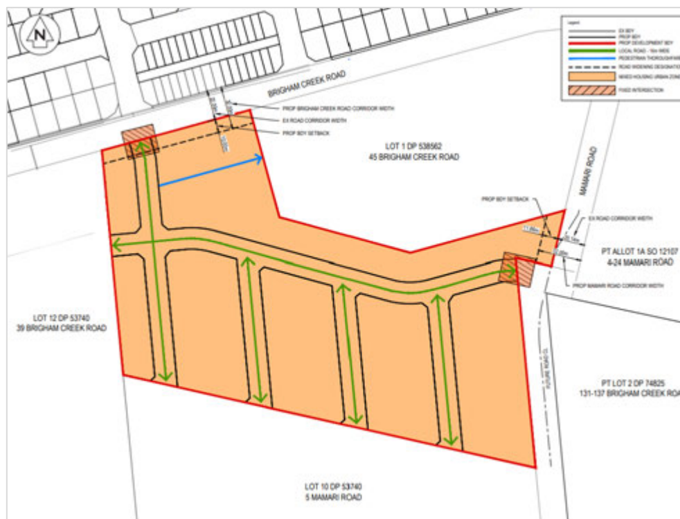
Figure 3: Plan to show proposed zoning, road layout, intersection points and designated area Source: Appendix 2 of Private Plan change request documentation
