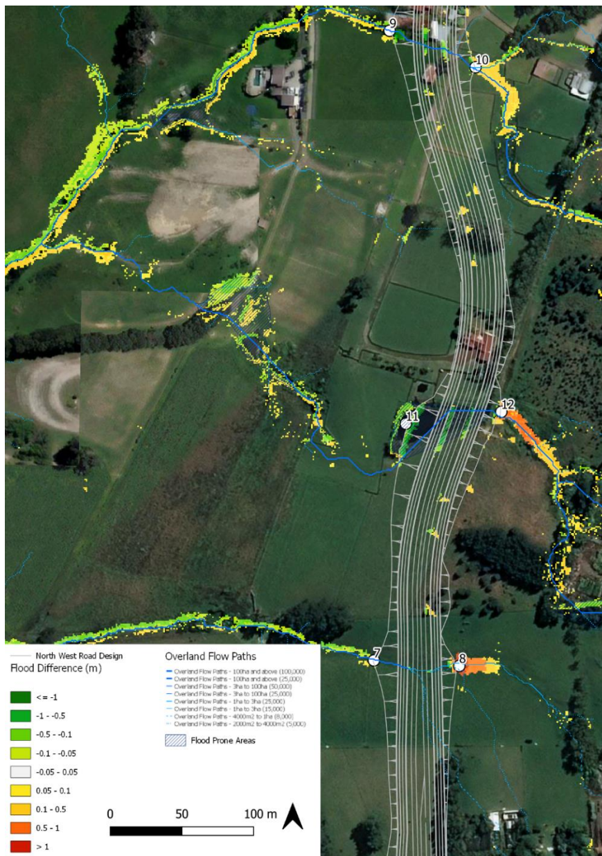
Figure 10-2: 100year flood difference map for Māmari Road (South)
