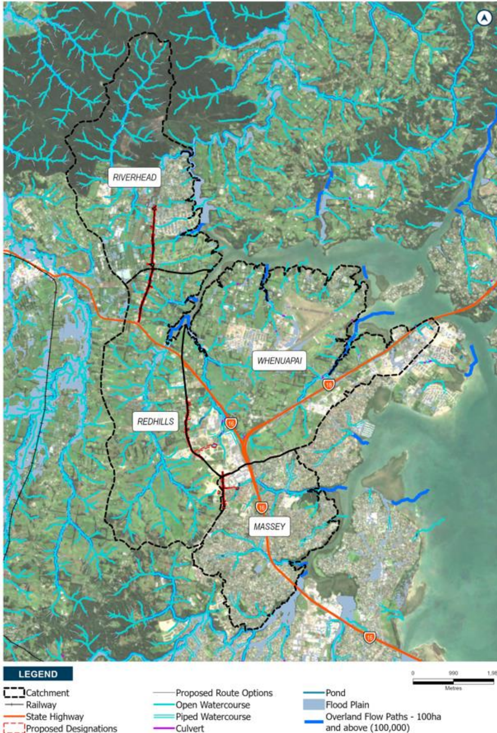
Figure 3-1: Existing 100 year ARI flood pain for Whenuapai, Massey, Riverhead and Redhills catchments (Auckland Council GIS)
