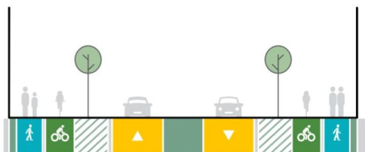
Figure 14-2: Coatesville-Riverhead Highway CFAF cross section outcome S1:SH16 to Short Road Indicative 24m cross section
