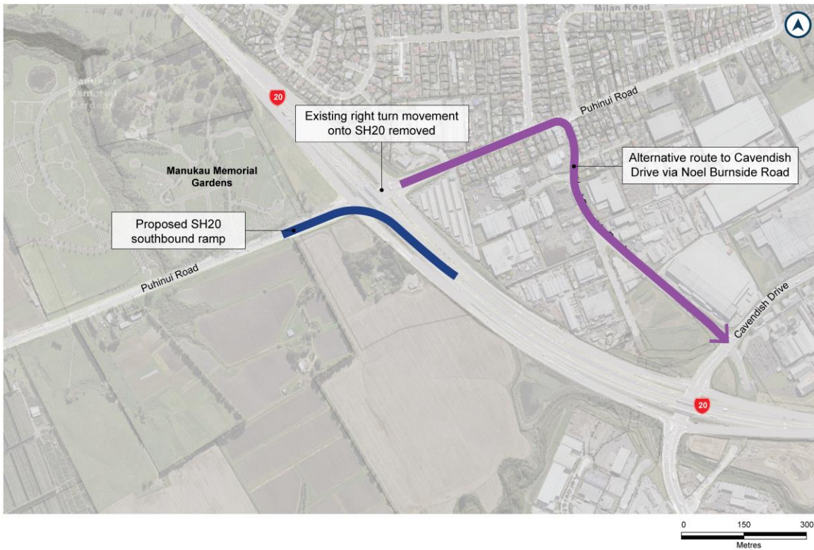
Figure 30: Change to SH20 southbound access
