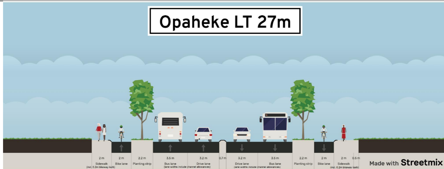
Figure 2: Opaheke Road, 27m cross-section (with four lanes, as proposed to be upgraded by others in future)
