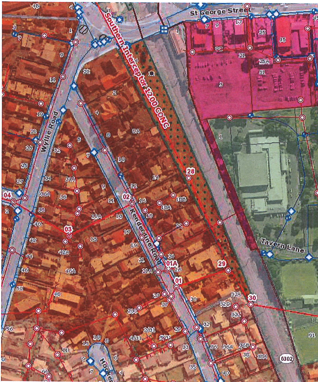
Figure 2: Southern Interceptor Wastewater Transmission Main at 12 Wyllie Road, Papatoetoe
