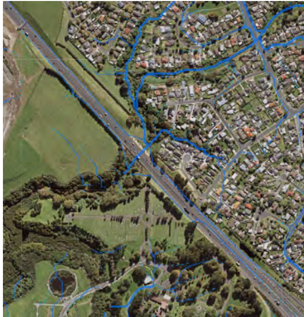
Figure 2-3: Example of Overland Flow Path shown as dashed ( 2000\text{m}^2 - 4000\text{m}^2 ), thin ( 4000\text{m}^2 - 3\text{ha} ) and thick ( >3\text{ha} ) blue lines according to the contributing catchment area.
