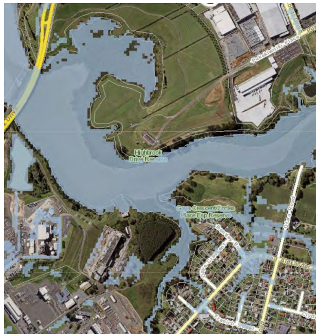
Figure 2-2: Example of Flood Plain shown as a semi-transparent light blue solid boundary.
