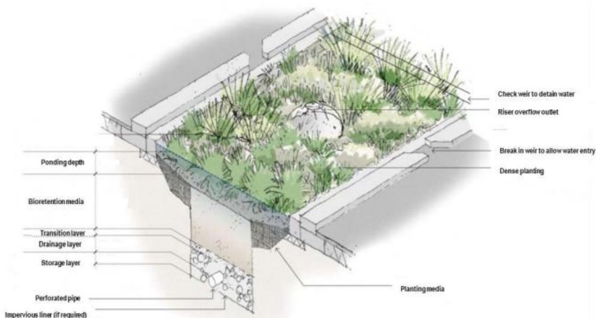
Figure 5: Schematic of bioretention swale (source: Auckland Council GD01)
