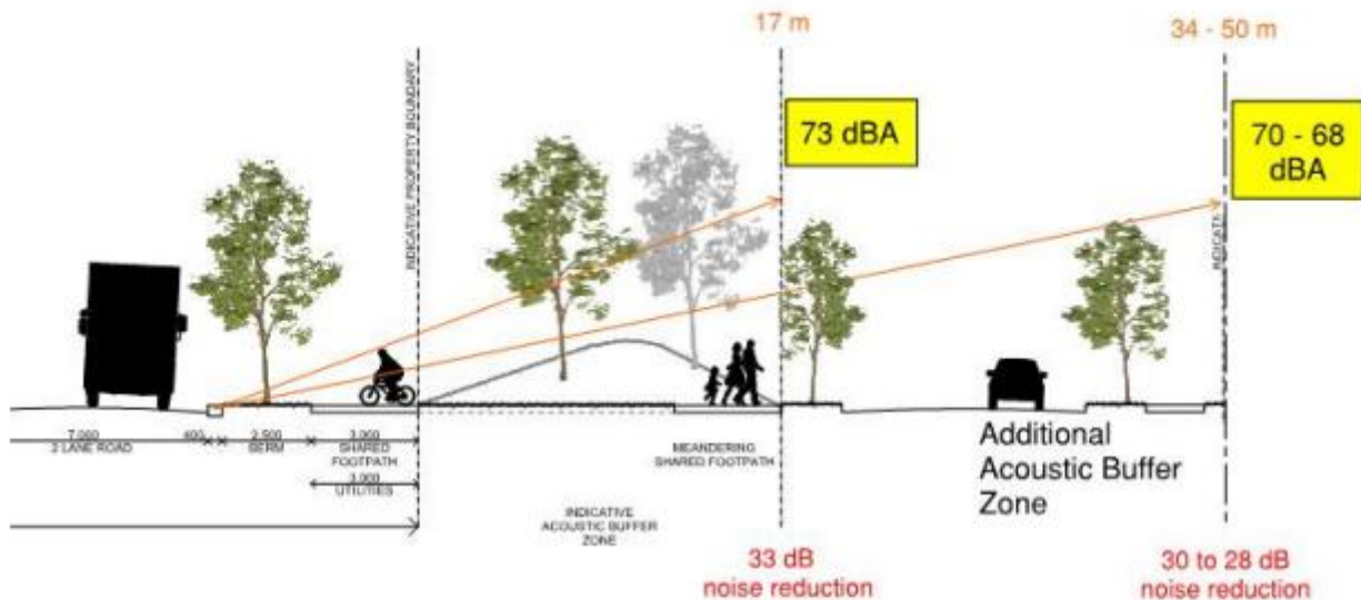
Figure 2: Indicative noise level based on existing typical road section
