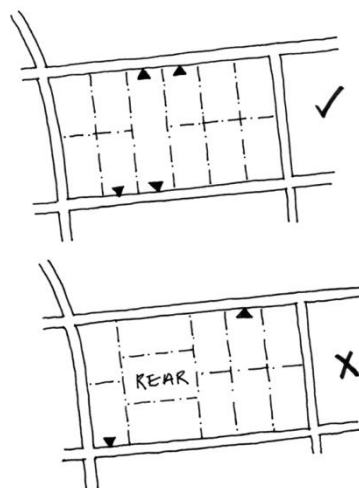
Diagram 4: All lots should front onto a legal road; through lots are permissible
