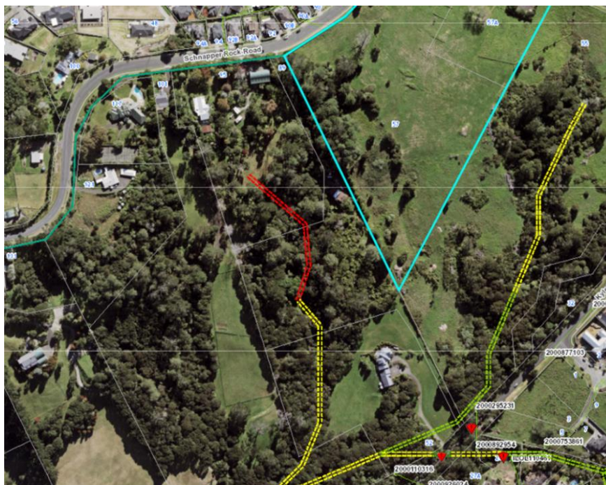
Figure 4. Stream erosion. Red line indicates erosion along the stream banks is greater than 60%, yellow indicated 20-40% bank erosion. Based on stream walkovers.
