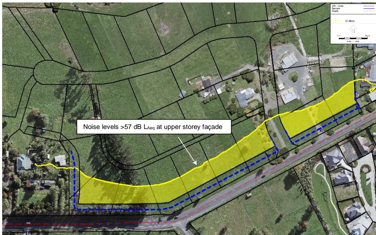
Figure 5: Noise levels at upper façade with 1.5 m high acoustic barrier on earth bund
