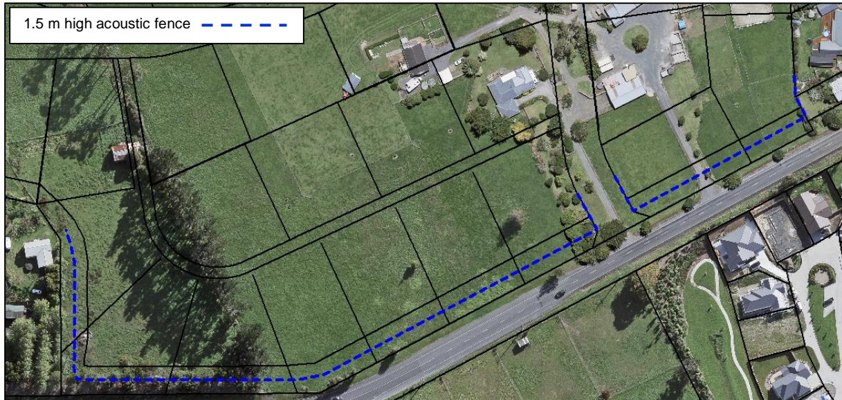
Figure 7: Extent of acoustic barrier
