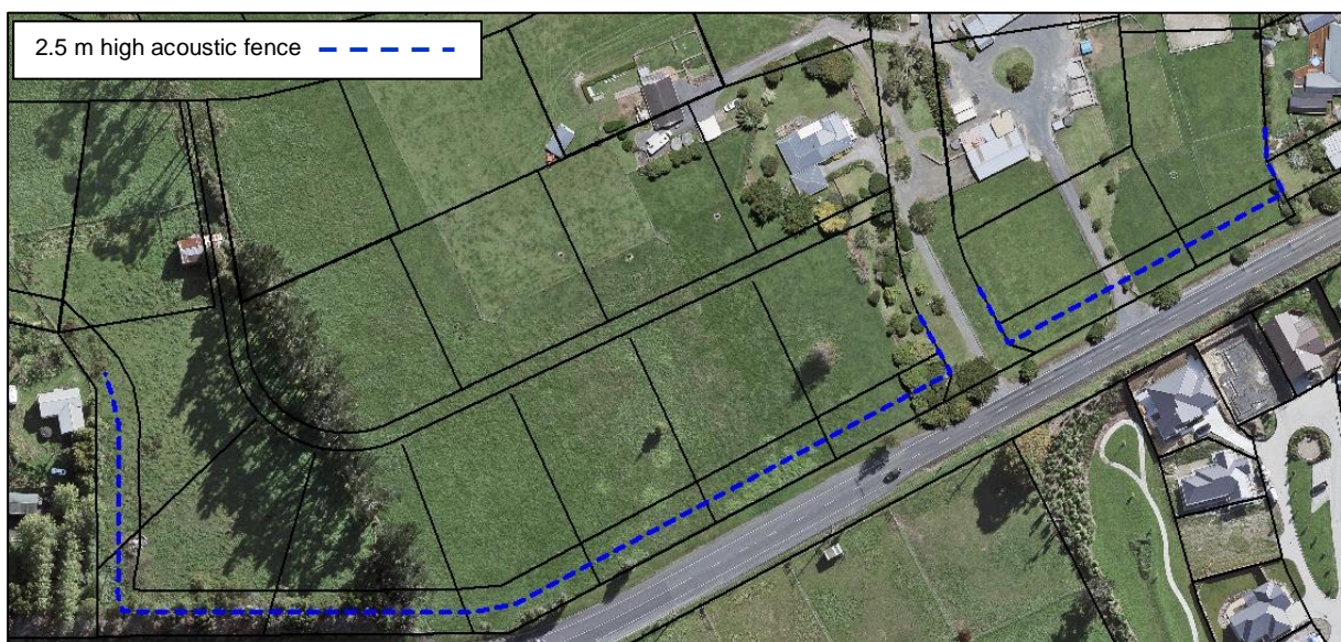
Figure 8: Extent of acoustic barrier
