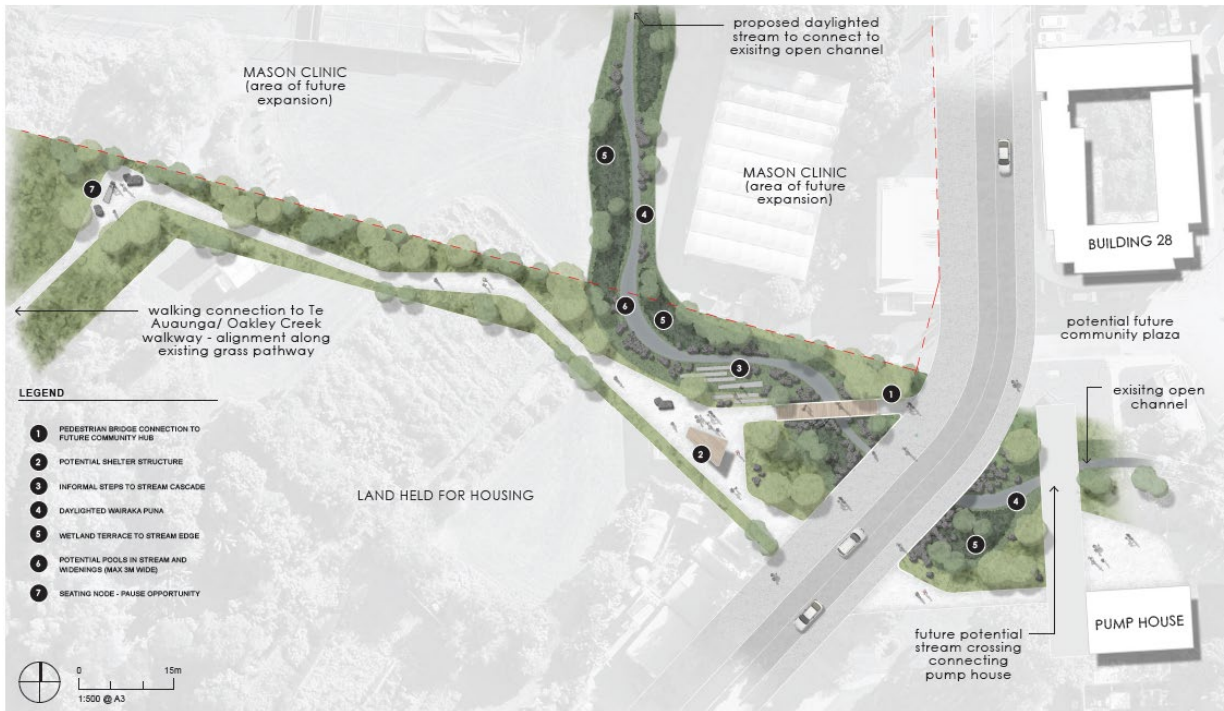
Figure 8: Landscape Plan for stream daylighting, showing walking path connection. Source: LUC60373078 approved plans, page 10.
