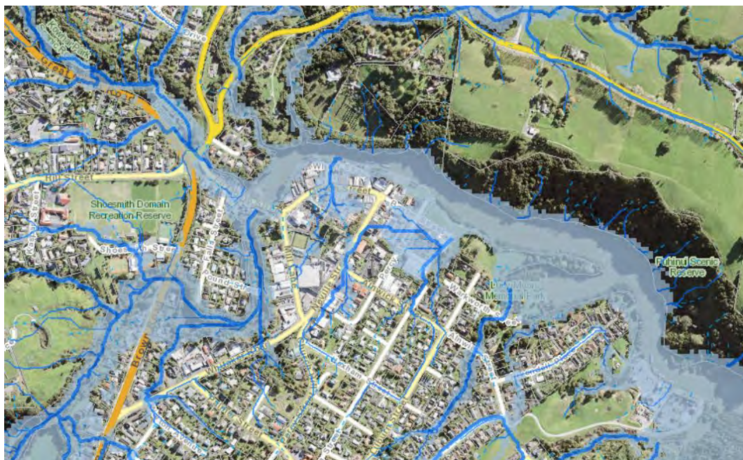
Figure 3. Auckland Council GeoMaps – Hill Road sub-catchment, existing flood hazards
