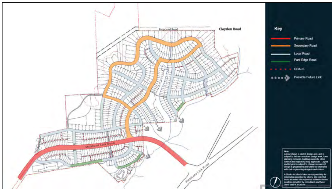
Figure 11: Potential Road Hierarchy Source: A Studio Architects
