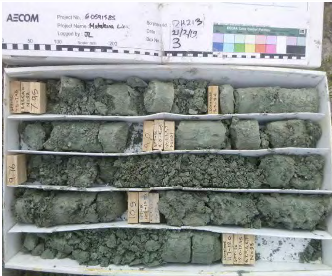
Box: 3 of 9 - Depth: 7.50m to 12.45m of 28.50m Date Drilled 20/02/2019 to 27/02/2019
