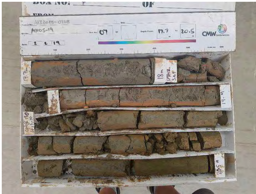
MH05-19: 17.7m to 20.5m
