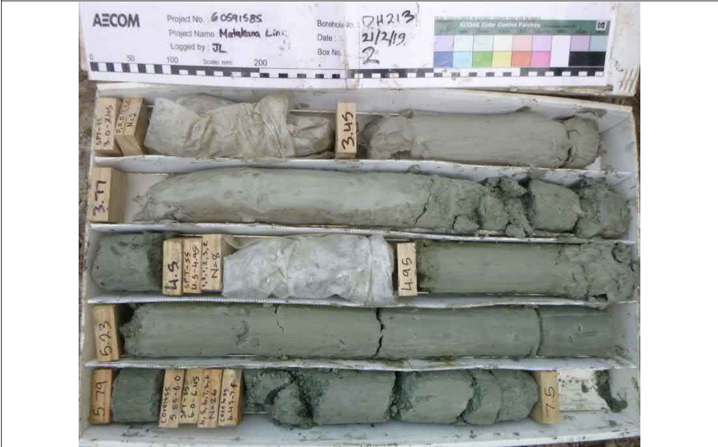
Box: 2 of 9 - Depth: 3.00m to 7.50m of 28.50m Date Drilled 20/02/2019 to 27/02/2019
