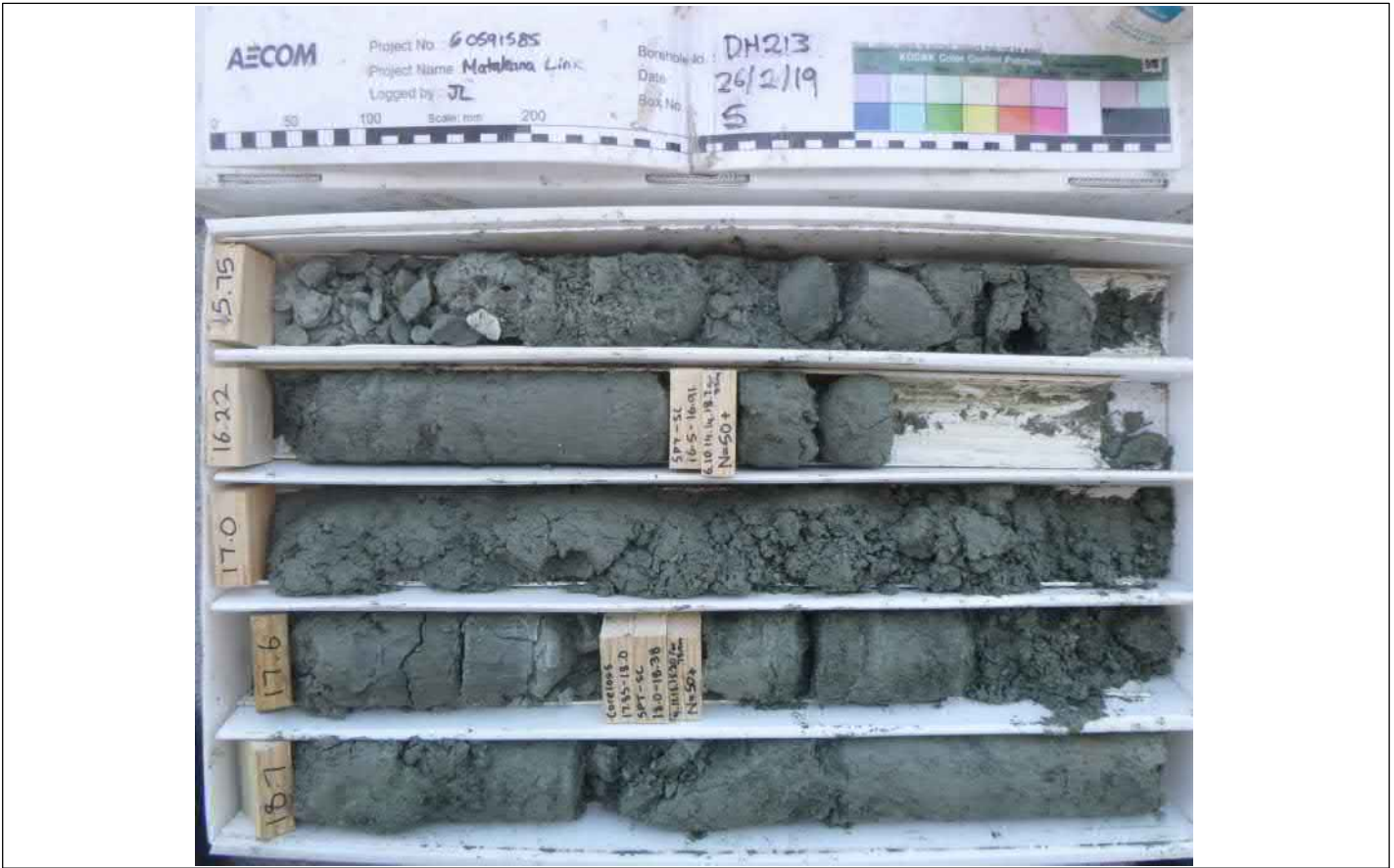
Box: 5 of 9 - Depth: 15.75m to 19.30m of 28.50m Date Drilled 20/02/2019 to 27/02/2019
