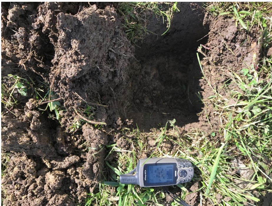
Figure 42. A test pit dug near the southern side of the stream, showing light brown topsoil onto a yellow clay base
