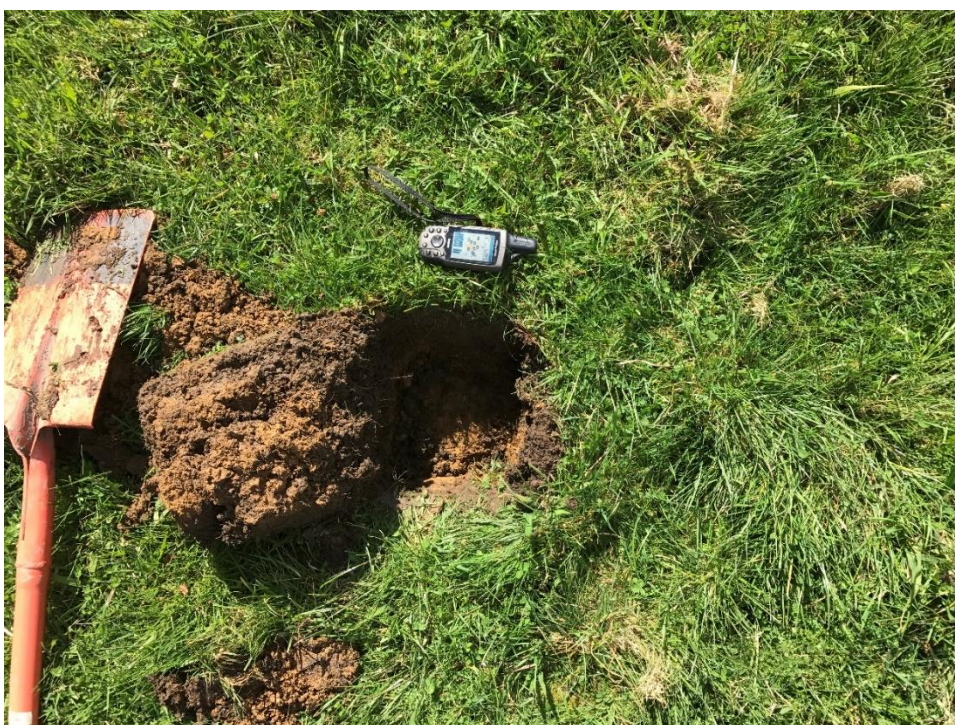
Figure 36. The test pit at the northern end of the proposed development area, near the river, showing light brown topsoil and a clay substrate
