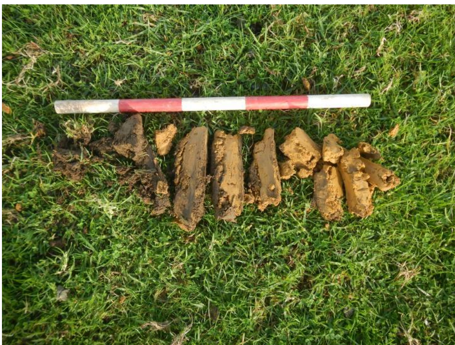
Figure 49. Example of hand auger results showing soil profile. The ranging pole is 50cm in length with 10cm intervals
