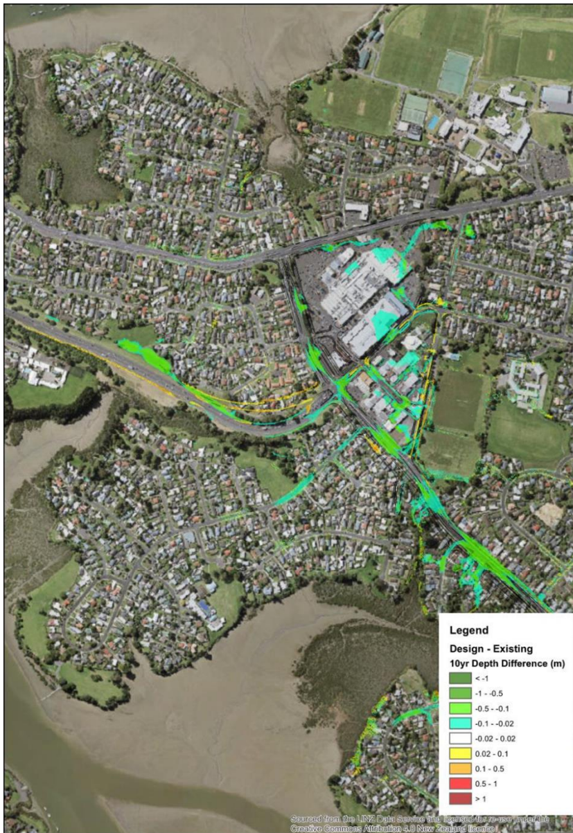
Figure 9-14 EB2 Design Case 10-Year Flood Depth Difference
