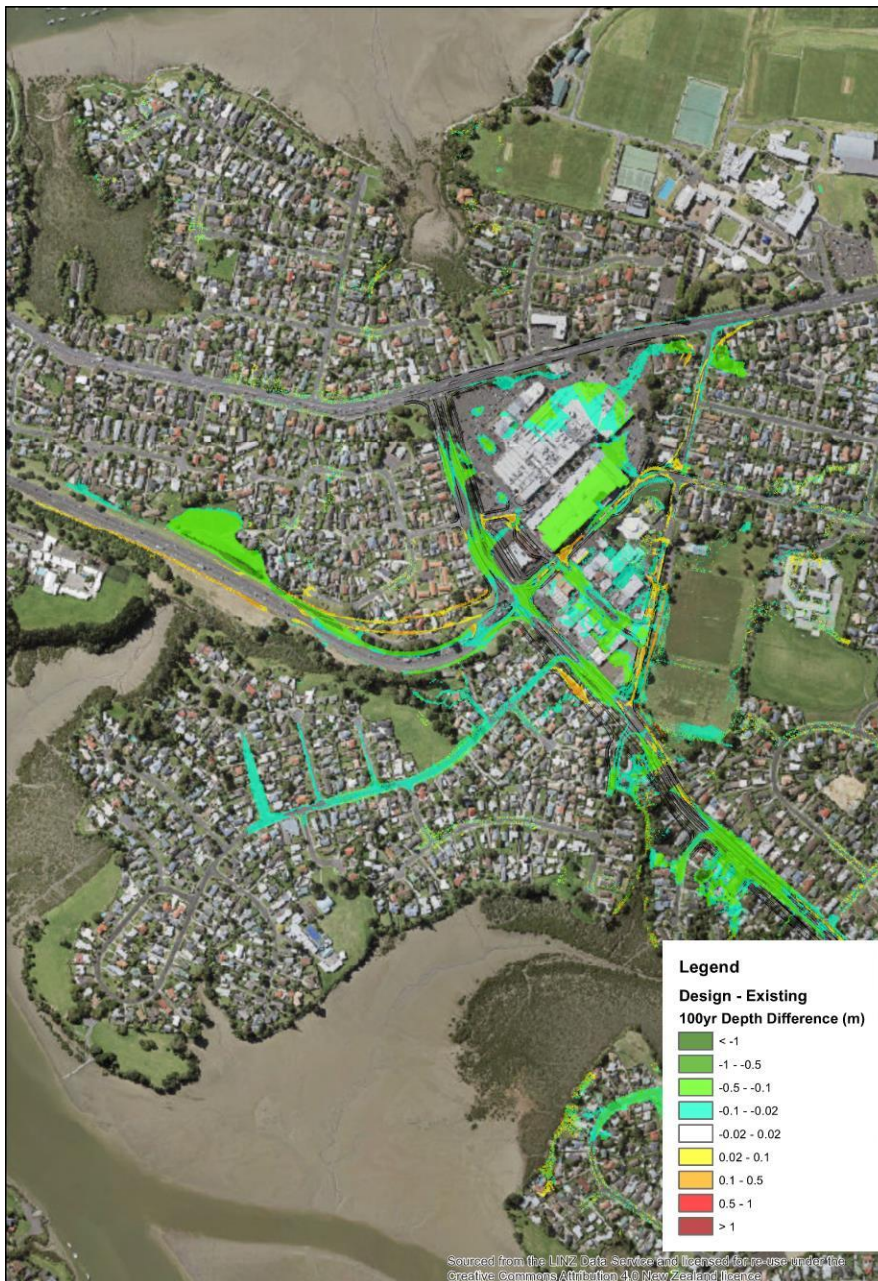
Figure 9-15 EB2 Design Case 100-Year Flood Depth Difference
