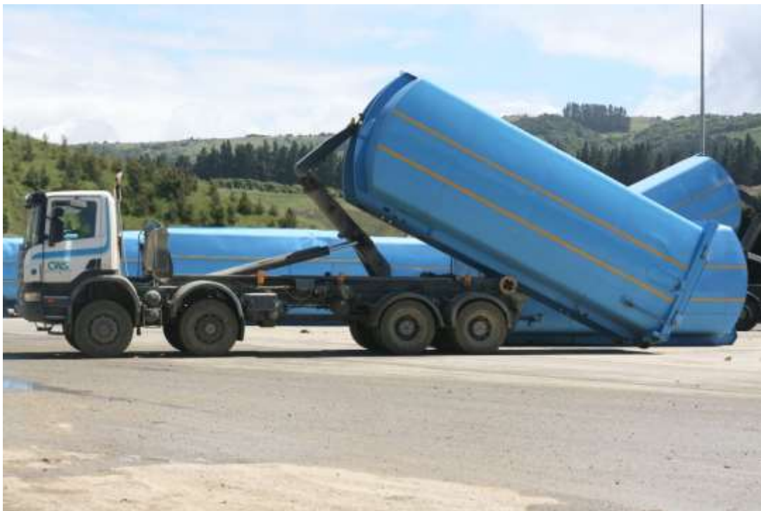
Figure 5.4: Mule truck at Kate Valley Landfill
