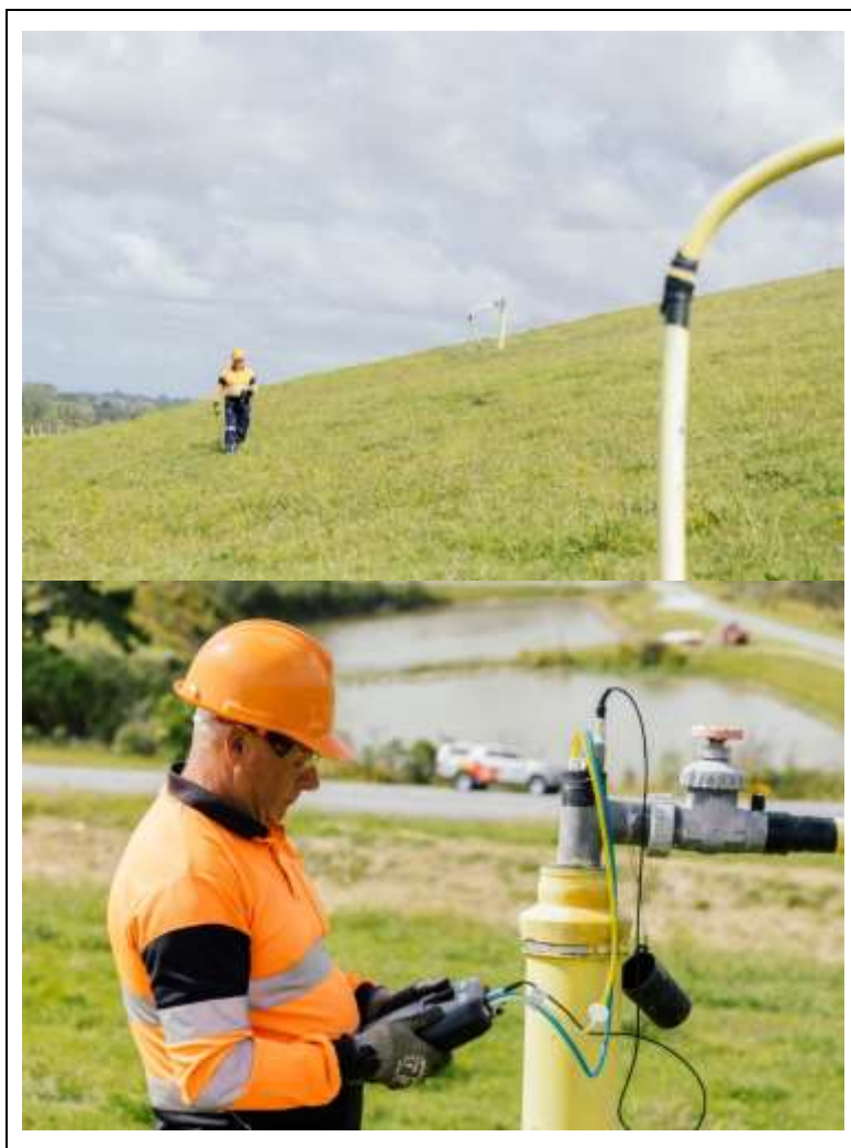
Figure 5.3: LFG monitoring wells at Redvale Landfill
