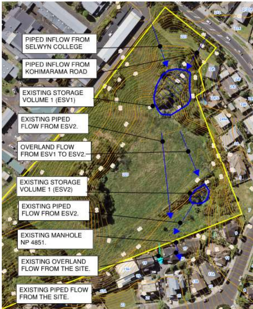
Figure 2.4 – Schematic Markup of Drainage Features through the Pre-development Site
