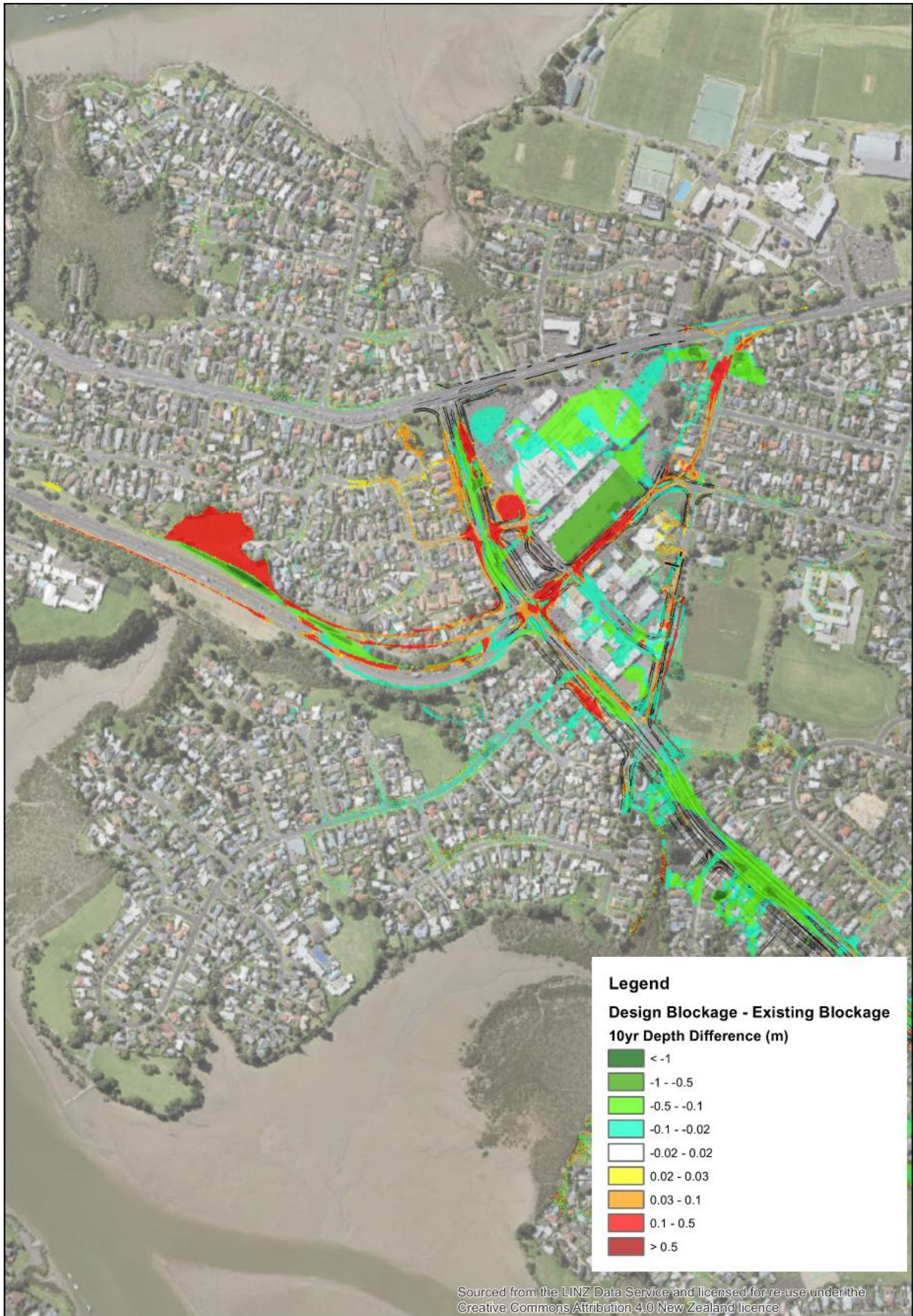
Figure 39: EB2 design case 10-year flood depth difference (pipe blockage)
