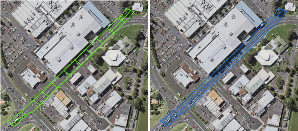
Figure 5: Flyover sub-catchments loaded to downpipes (green) and flyover sub-catchment to be loaded to the pipe network to the west in the detailed design stage (blue).
