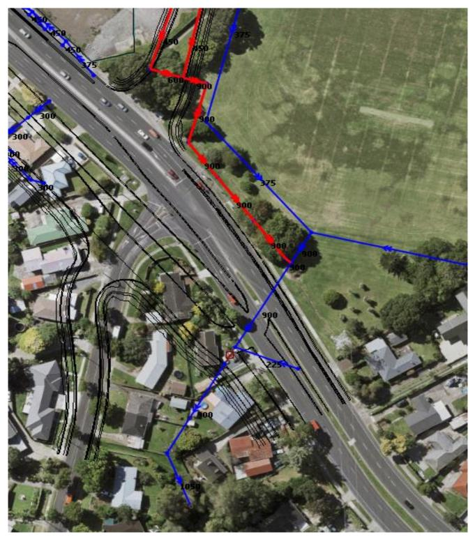
Figure 12: WRR design network highlighted in red connecting to the existing pipe network shown in blue.
