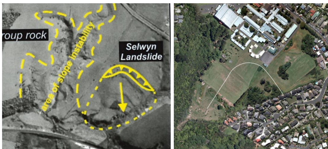
Appendix Figure B: Mapped extent of the Selwyn Landslide, shown on left from 1999 thesis 8 and overlain on 2017 aerial on image on right, the back scarp is shown by the white line.
