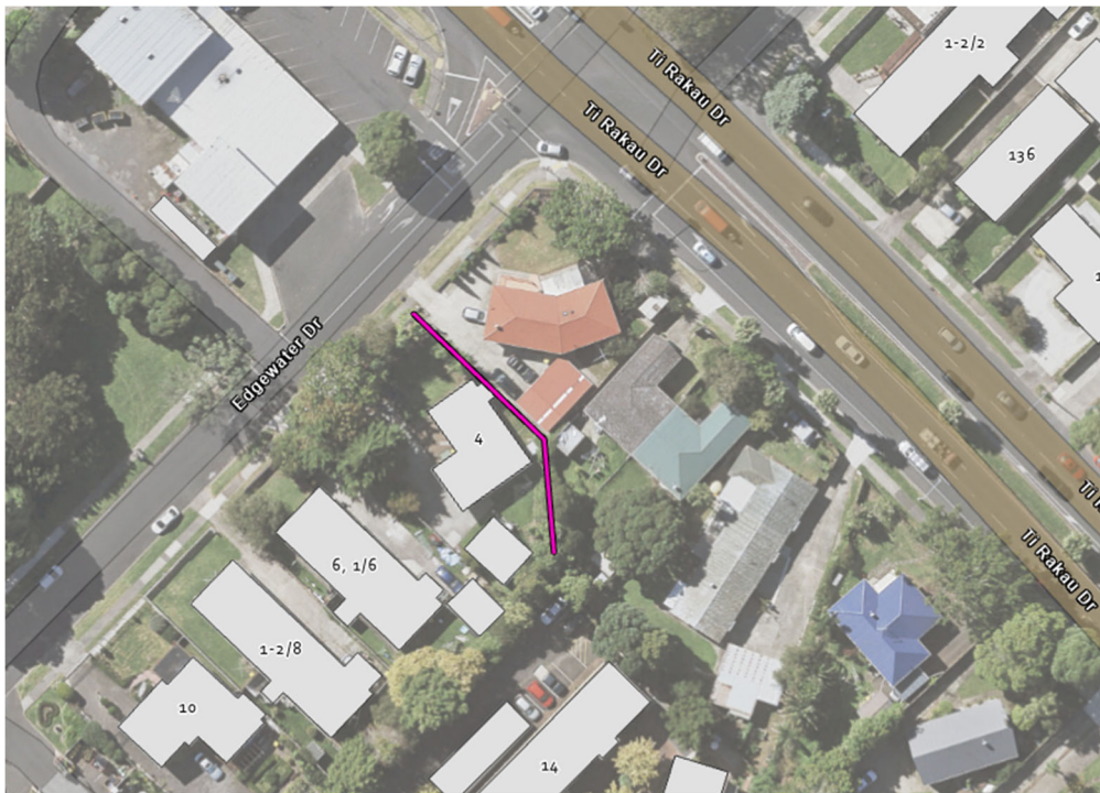
Figure 5 Proposed noise wall location - 4 Edgewater Drive
