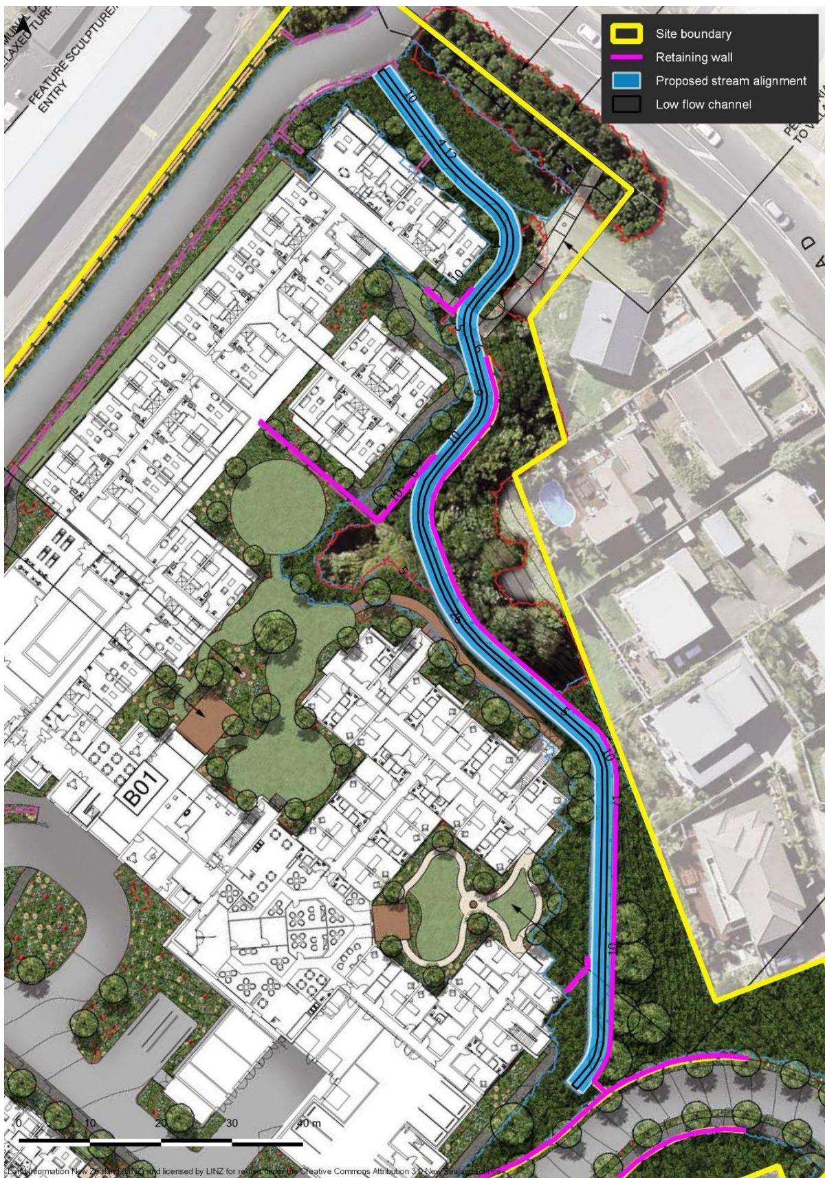
Figure 10: Proposed stream alignment and planting (plan from Design Squared).
