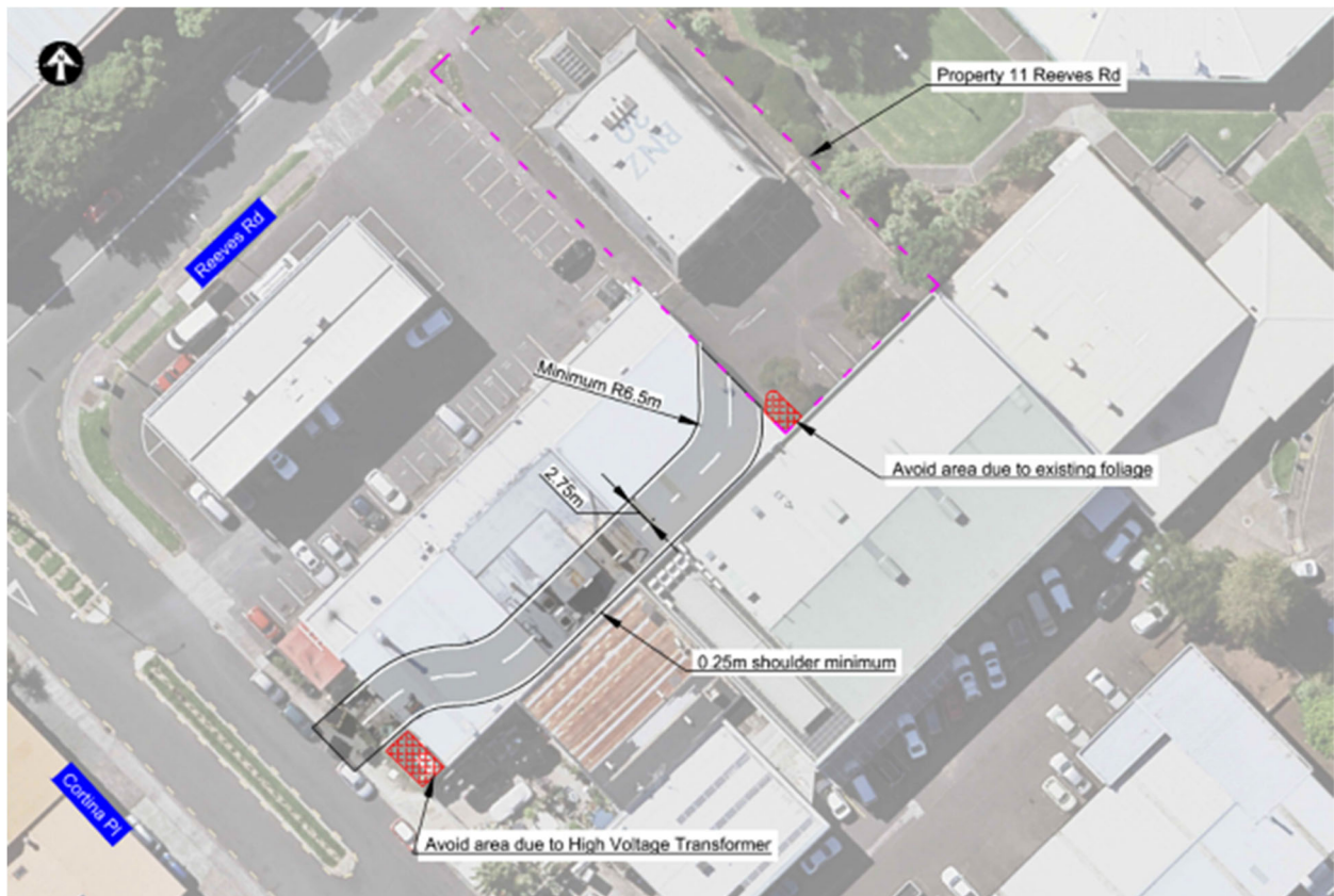
Figure 79: 11 Reeves Rd temporary access during construction
