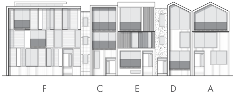
Figure A2.4 How variation occurs with further mix and match of facades, including a 'double width' dwelling (type F).
