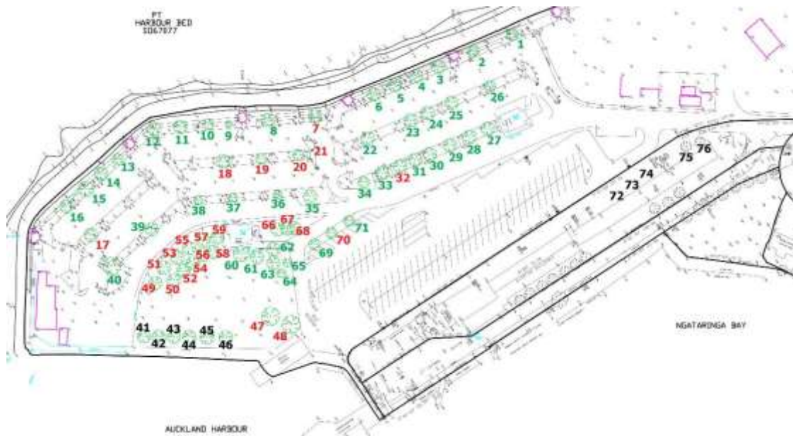
Figure 1 – screenshot of the Tree Location Plan. Green numbers indicate potential transplant specimens, red – those that are not suitable, and black - trees that will be retained and protected in situ
