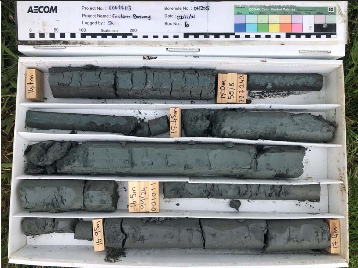
Box: 6 of 11 - Depth: 14.70m to 17.40m of 28.00m Date Drilled 1/11/2021 to 24/11/2021 - Date Photographed: 2/11/2021
