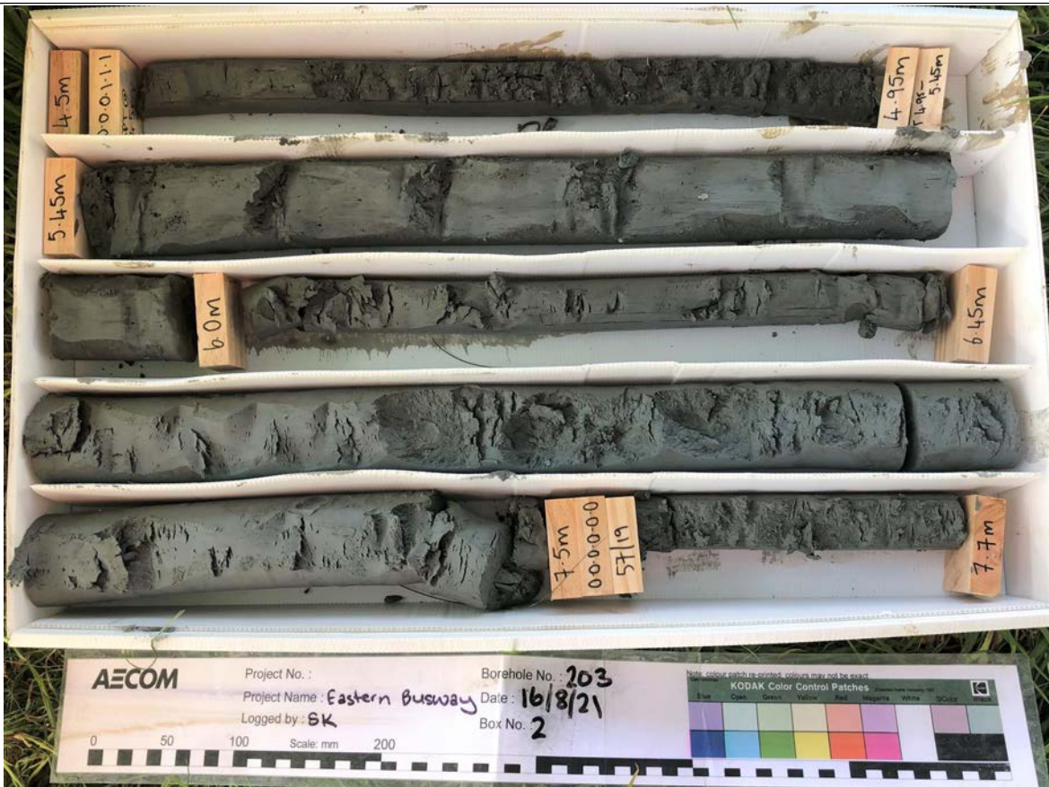
Box: 2 of 8 - Depth: 04.50m to 07.70m of 24.00m Date Drilled 16/08/2021 to 17/08/2021 - Date Photographed: 16/08/2021
