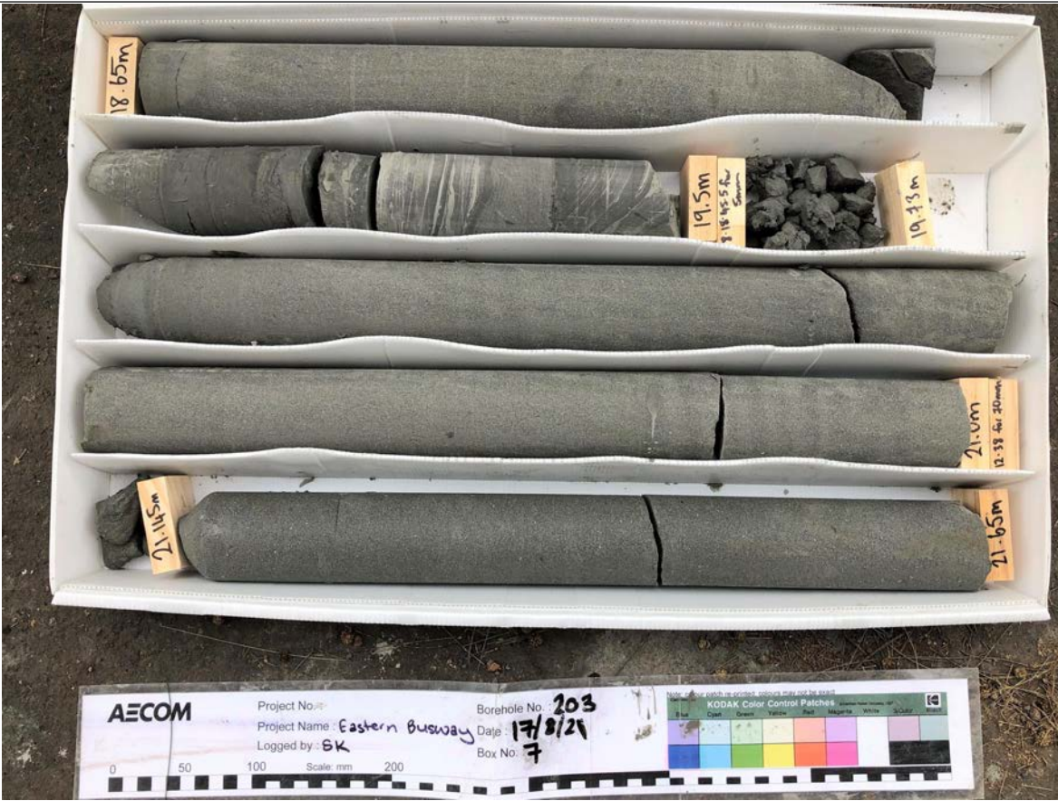
Box: 7 of 8 - Depth: 18.65m to 21.65m of 24.00m Date Drilled 16/08/2021 to 17/08/2021 - Date Photographed: 17/08/2021
