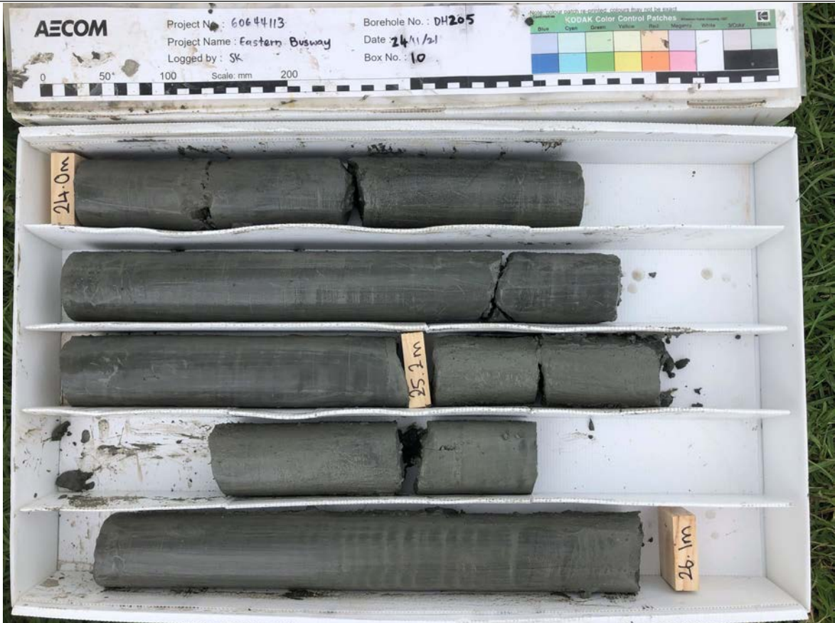
Box: 10 of 11 - Depth: 24.00m to 26.10m of 28.00m Date Drilled 1/11/2021 to 24/11/2021 - Date Photographed: 24/11/2021
