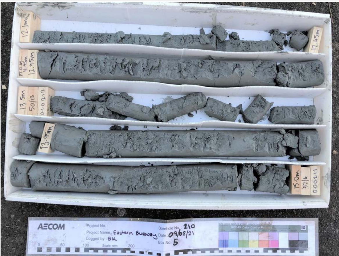
Box: 5 of 12 - Depth: 12.10m to 15.00m of 33.00m Date Drilled 6/08/2021 to 10/08/2021 - Date Photographed: 9/08/2021
