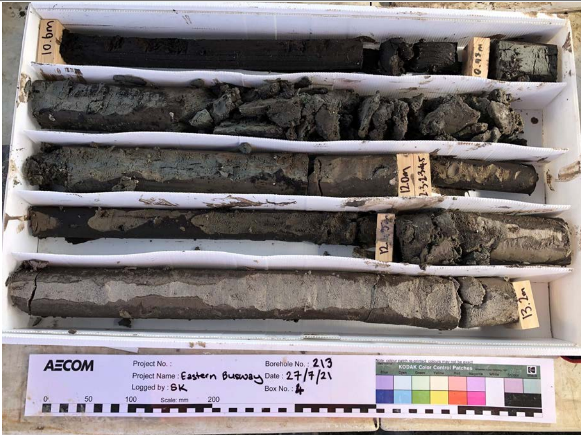
Box: 4 of 13 - Depth: 10.60m to 13.20m of 35.00m Date Drilled 27/07/2021 to 28/07/2021 - Date Photographed: 27/07/2021
