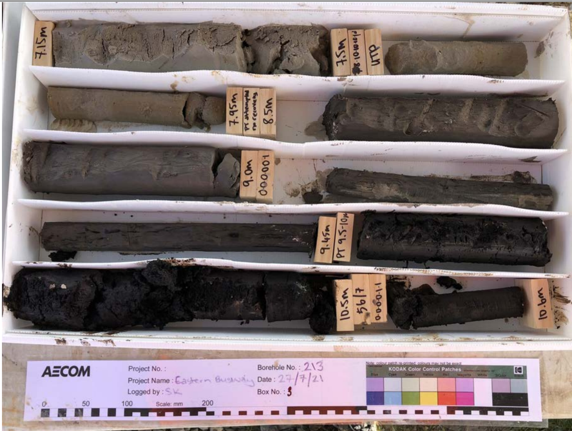
Box: 3 of 13 - Depth: 07.15m to 10.60m of 35.00m Date Drilled 27/07/2021 to 28/07/2021 - Date Photographed: 27/07/2021
