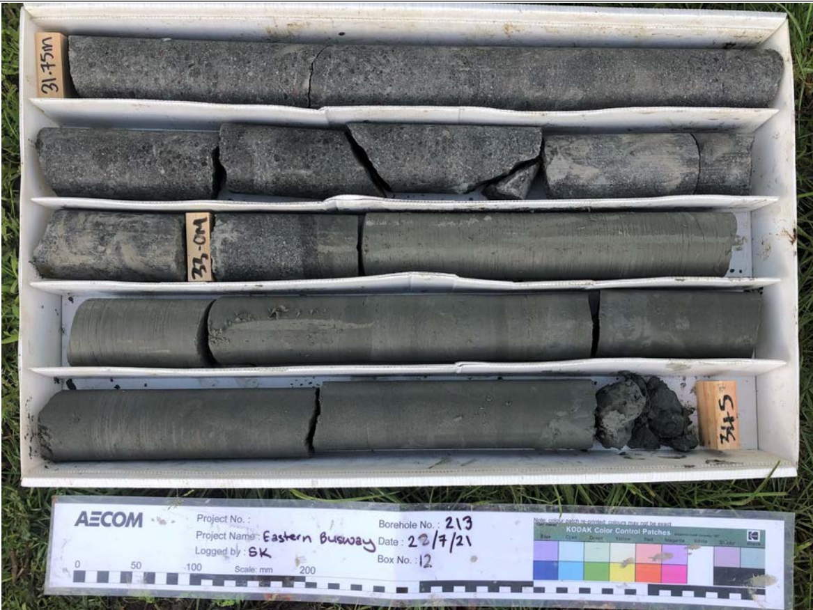
Box: 12 of 13 - Depth: 31.75m to 34.50m of 35.00m Date Drilled 27/07/2021 to 28/07/2021 - Date Photographed: 28/07/2021
