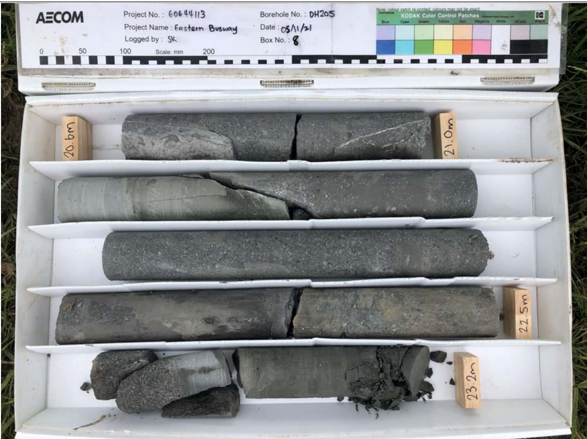
Box: 8 of 11 - Depth: 20.60m to 23.20m of 28.00m Date Drilled 1/11/2021 to 24/11/2021 - Date Photographed: 5/11/2021
