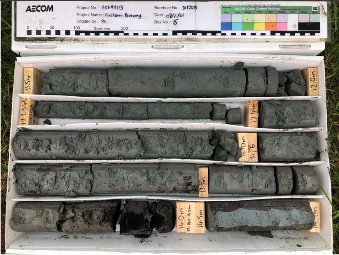
Box: 5 of 11 - Depth: 11.50m to 14.70m of 28.00m Date Drilled 1/11/2021 to 24/11/2021 - Date Photographed: 2/11/2021
