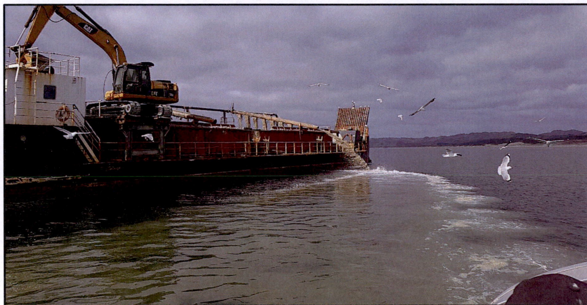
Figure 5.1 Sand barge in operation showing discharge of material, turbid plume and birds foraging.
