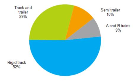
Note: A Train: A towing vehicle with a semi-trailer followed by a full trailer.
