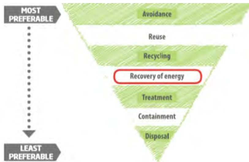
Figure 2: Waste Hierarchy showing the order of preference and where EfW is placed (Environment Protection Act 1970, p.4)
