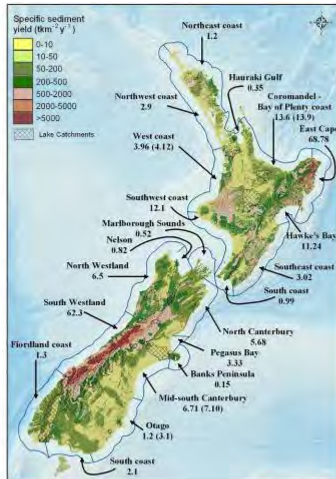
Figure 3: Annual present-day suspended sediment yields into different coastal areas of New Zealand. Numbers given are tonnes x 10 6 per year; bracketed figures are predicted yields if rivers had no dams on them. (Source: Murray Hicks, NIWA.)
