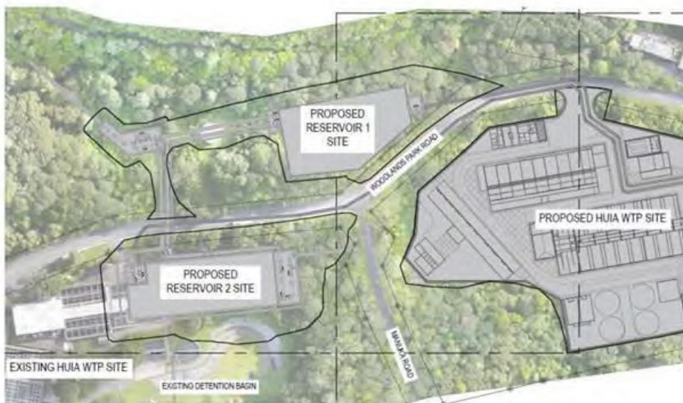
Figure 4 Proposed Huia Reservoir Site Layout (now revised - Refer Reservoir Site Layout Development Report, Beca, May 2019)
