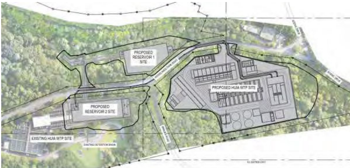
Figure 1 - Construction footprints (solid black outline) and indicative layouts of the proposed replacement WTP and reservoirs
