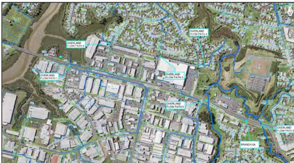
Figure 6-12 EB3C existing overland flow paths
