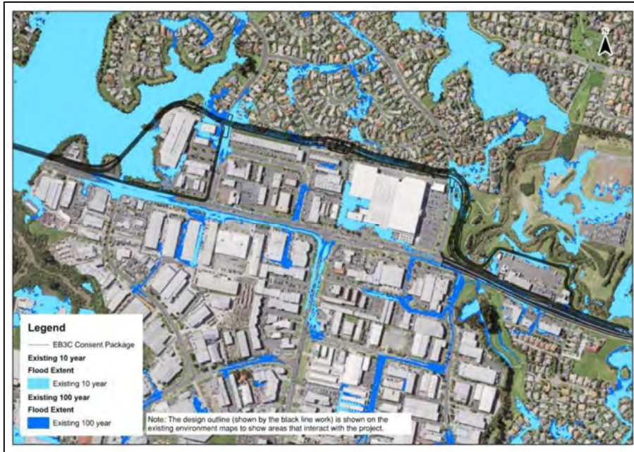
Figure 6-13 EB3C Base Case 10 and 100-year Flood Extents
