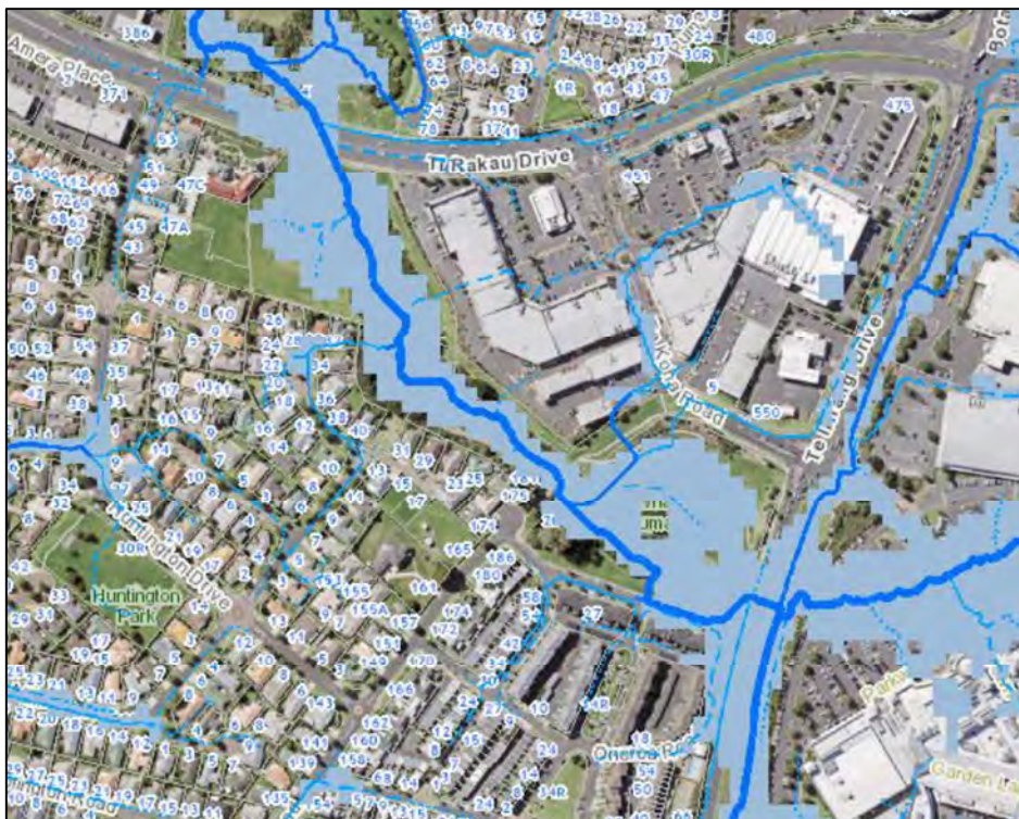
Figure 6-14 EB4L Existing 100-year Flood Extents (sourced from Auckland Council Geomaps)
