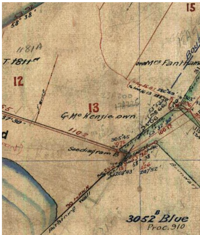
Figure 13. DP 12834 (1919) showing the land taken for the submarine mining base (bounded by the retaining wall), and the top of the escarpment at the rear of the property (irregular red line).
