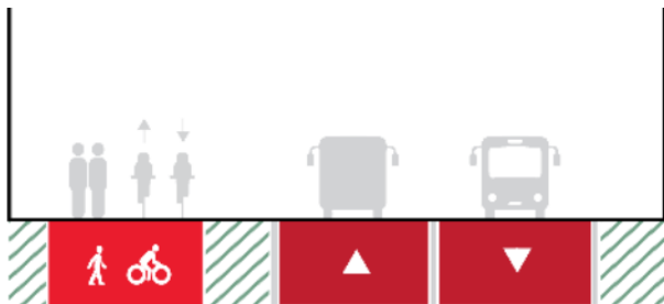
Figure 10-17: Typical Cross Section – RTC alongside ASH at Taupaki Road (shared path will re-join RTC at Boord Crescent)
