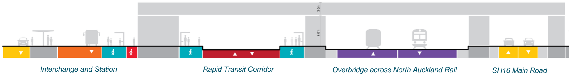
Figure 10-22: Huapai Station indicative cross section (including overbridge across NAL and SH16 to southern side)
